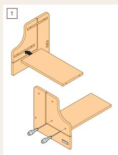
Hold one of the two side boards and attach the lower step (the one that doesn't have a handle hole) to it with two bolts using a screwdriver. Do not tighten the bolts at this step.
