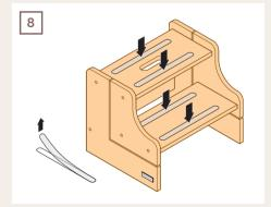
Optionally, install the anti-slip stickers: two on the lower step, and two on the upper step. Remove the protective layer from the stickers.
