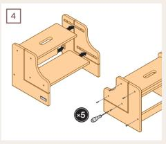
Attach the other side board to the two two steps (with two bolts for each) and to the support beam (with one bolt). At this step, you can tighten the bolts, but make sure not to overdo it: stop when you feel resistance.
