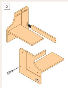
Attach the support beam to the side board with one bolt. Do not tighten the bolt.
