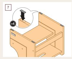
Flip the stool upside down and attach the four anti–slip pads to the bottom.
