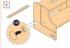
Stick the bolt covers onto the bolt heads all around the stool.
