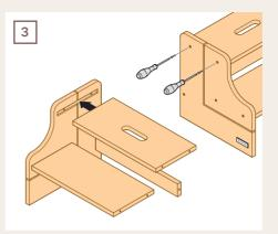
Attach the upper step (the one that has a handle hole) to the side board with two bolts. Do not tighten the bolts.
